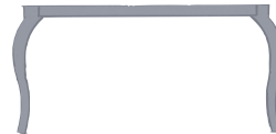
Coffee Table 25" W x 47" L x 17" H 28" W x 50" L outside dimension of cabriole leg
